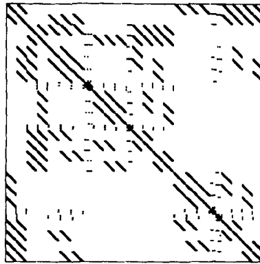
Figure 8. Sparsity pattern P_0 corresponding to an irregular numbering of nodes in the mesh used for Figure 6; 4921 non-zeros
